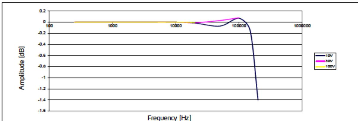
The Frequency response for the 0 VDC and 200 VDC outputs, 3 meter RG-58 cable, 10, 30 and 100 V RMS.
