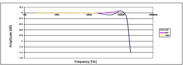
The Frequency response for the O VDC and 200 VDC outputs, 3 meter RG-58 cable, 10, 30 and 100 V RMS.
