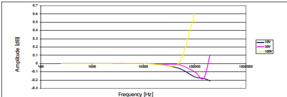
The Frequency response for the 0 VDC and 200 VDC outputs, 1 meter RG58 cable, 10, 30 and 100 V RMS.
