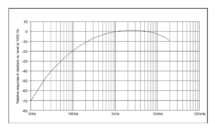
Frequency response of A-weighting filter (compliant with IEC 61672-1 Class 1)
