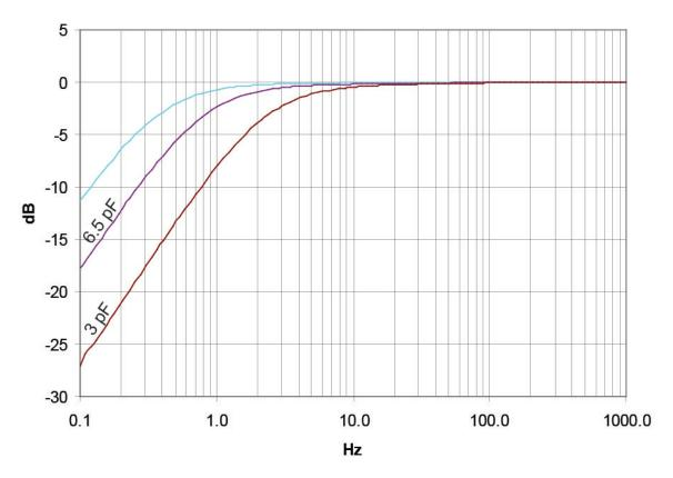
Typical low-frequency response of Type 26AL for  $\frac{1}{2}$  (20 pF),  $\frac{1}{4}$  (6.5 pF) and  $\frac{1}{6}$  (3 pF) microphones
