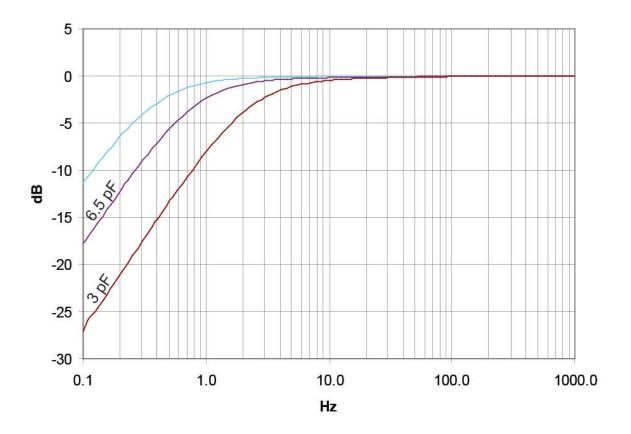
Typical low-frequency response for  $\frac{1}{2}$  (20 pF),  $\frac{1}{4}$  (6.5 pF) and  $\frac{1}{6}$  (3 pF) microphones
