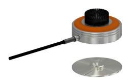
When the microphone is placed over the mounting disc, a center guide ensures that the microphone will be attached and centered to the disc correctly once the magnetic force kicks in. In this way, it is easy to mount in difficult-to-access locations with no loss of placement accuracy.
