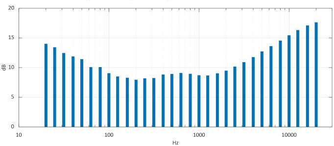
Typical noise spectrum (Typical A-weighted level = 23.5 dBA)
