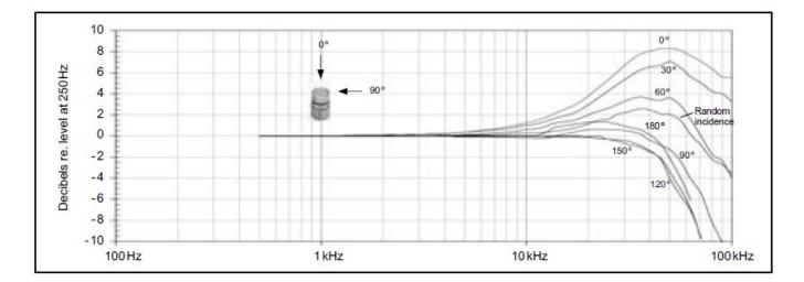
Free-field corrections for different angles of incidence
