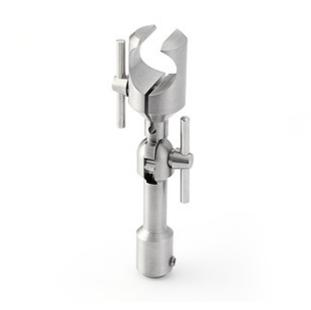
Material: Stainless steel Dimension: For 1/2" Special feature: Adjustable in 45 degree steps The GRAS RA0093 is an adapter for mounting a microphone set (microphone/preamplifier) on tripods having a standard 1/4" UNC-20 male thread. The adapter is provided with a clamp for attaching a 1/2" diameter preamplifier. The microphone can be set in angles between 0 and 180 degrees in 45 degree steps.
