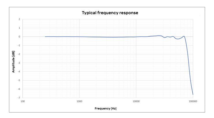
The frequency response is within ±3 dB up to 70 kHz
